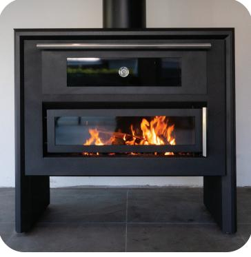
**FIREBOX** 100W X 30D X 38H CM **MATERIAL** 3-6MM STEEL **FINISH** METALLIC BLACK PAINT **OVEN VOLUME** 58 I TR OVEN 69W X 43D X 18H CM **OPEN COAL VOLUME** 136 LTR **MAX LOG** 220 X 85L CM **BAFFLES & DOORS** STEEL **HEAT BANKS** CERAMIC PLATE **SPIGOT FULLY WELDED**
